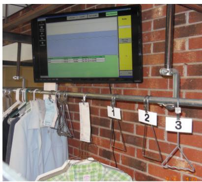
Fabricare Assembly Manager is user-friendly and works by simply scanning unique barcodes that were heat-sealed into garments at mark-in. Once a garment is scanned in the assembly bay, the screen will show you in a large font the slot number to hang the garment. If being used, the speakers or headphones will also tell you where to hang the garment at the same time.
